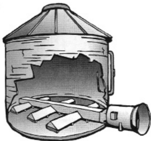
Figure 5.2 Grain storage recirculation system
