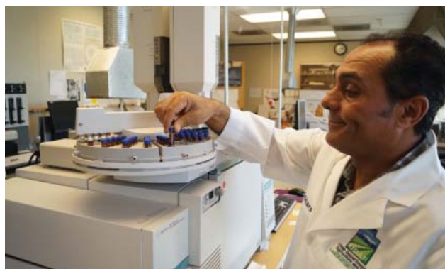
Chemist/Lab Manager, Mohammed Sharaf, Conducting a pesticide residue test using a GC/MS Gas Chromatography mass chromatography.
